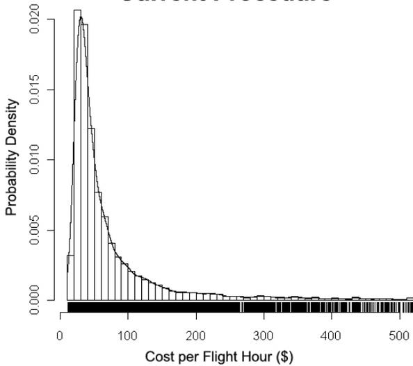
**Figure 3 — The uncertainty distribution for  $C_{fis}$ , the cost of maintenance per flight hour allowing the turbine to fail in service, shows appreciable risk at very large cost per flight hour values.**
