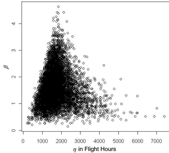
**Figure 2 — The 10,000 joint samples of  $\eta$  and  $\beta$  obtained using a Markov Chain Monte Carlo process based on the five failure and one survivor data show a non-intuitive joint distribution.**
