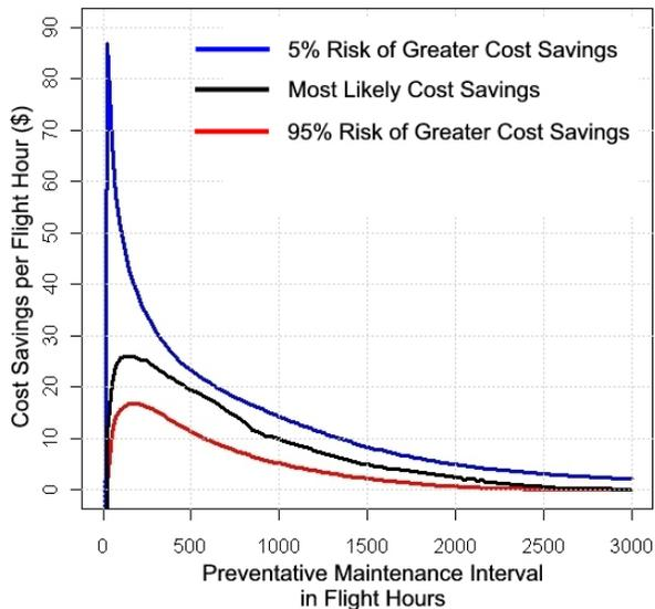
**Figure 6 — The risks for cost savings per flight hour using a preventative maintenance interval show peaks at all risk levels for preventative maintenance intervals between 50 and 350 flight hours, the same region for the minima in Figure 5.**
