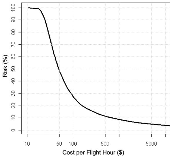
**Figure 4 — Based on the available data, there is a 50% risk that maintenance cost will exceed \$49 per flight hour when the turbine is allowed to fail in service.**
