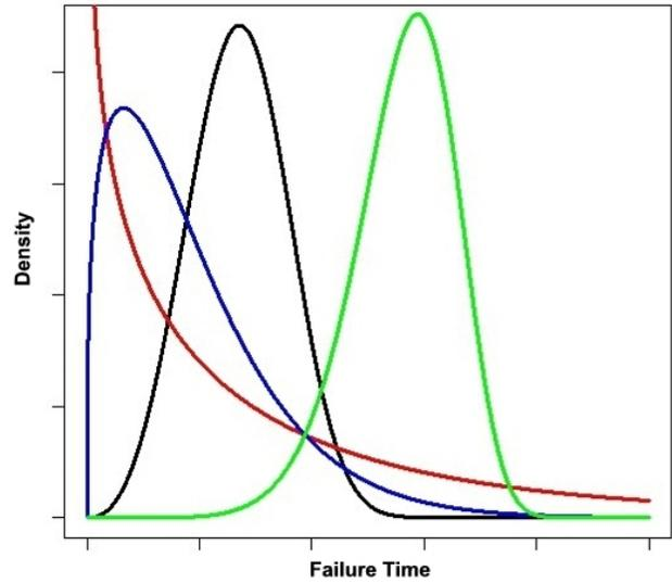
**Figure 1 — Being the most general of the one-sided uni-modal uncertainty models, the Weibull model provides a wide variety of shapes for failure time models.**
