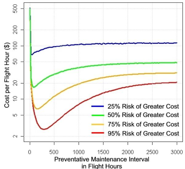
**Figure 5 — Preventative maintenance costs appear to be minimal at all risk levels for preventative maintenance intervals between 50 and 350 flight hours.**
